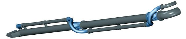
Gimbal Replacement Hoses are special designed hoses to replace the steel construction of gimbals and universal joints general build into a drag arm to allow the required flexibility. The design incorporates flexibility as well as lateral rigidity to minimize the offset of the single pipe section. Tensile breaking strength is designed as high to achieve the necessary strength required within a drag
