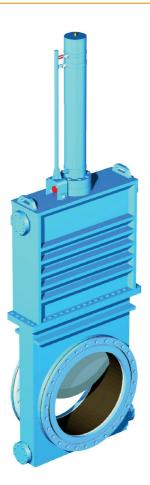
EMSTEC Gate valves are linear motion valves in which a flat closure element slides into the flow stream to provide shut-off. Gate valves are designed to minimize pressure drop across the valve in the fully opened position and stop the flow of fluid completely. The direction of fluid flow does not change, and the diameter through which the process fluid passes is essentially equal to that of the pipe. Hence, have minimal pressure drop when opened fully.
