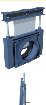
EMSTEC Shore valves are linear motion valves in which a flat closure element slides into the flow stream to provide shut-off. Shore valves are designed to minimize pressure drop across the valve in the fully opened position and stop the flow of fluid completely. The direction of fluid flow does not change, and the diameter through which the process fluid passes is essentially equal to that of the pipe. Hence, they have minimal pressure drop when opened fully.
